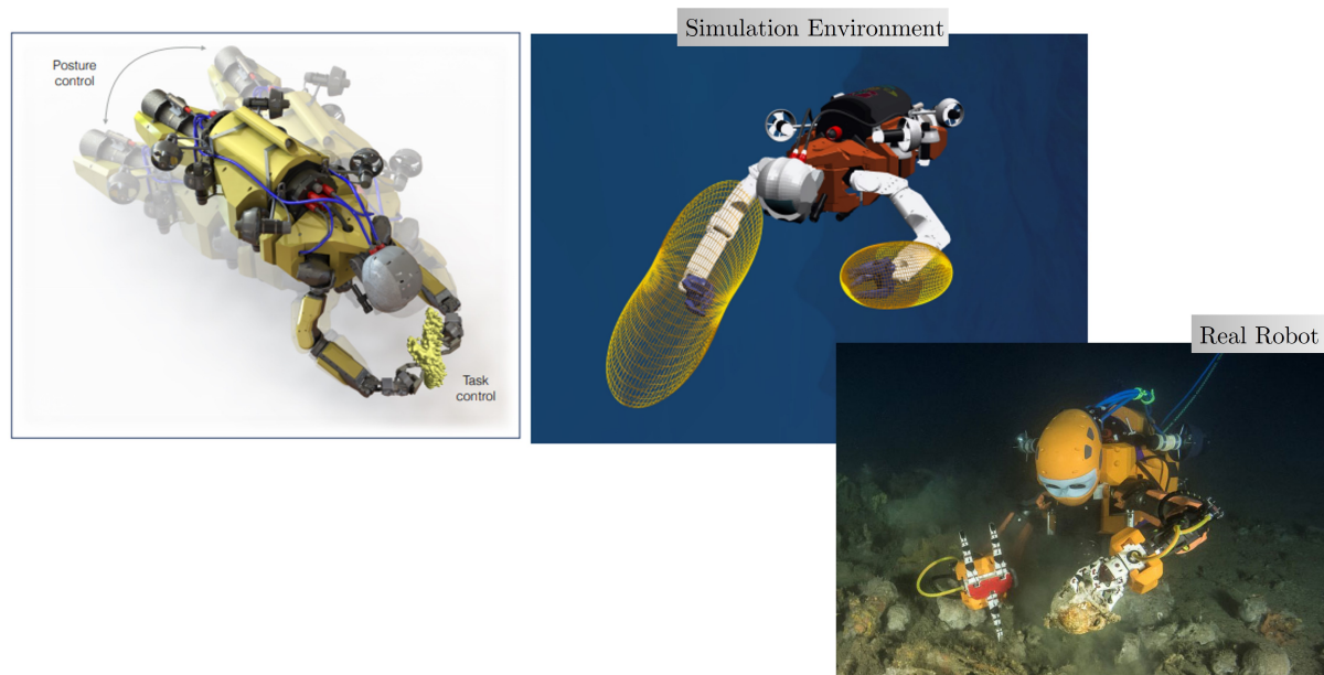
Figure 4 – Simulation and experiment: Ocean One control of posture. The deployment in the experimental field of Ocean One: its maiden mission to the Lune (Louis XIV’s two-decked, 54-gun flagship that sunk in 1664 off the coast of Toulon, France), where it inspected the ship remnants and recovered an archeological artifact (BRANTNER; KHATIB, 2021; KHATIB et al., 2016).
