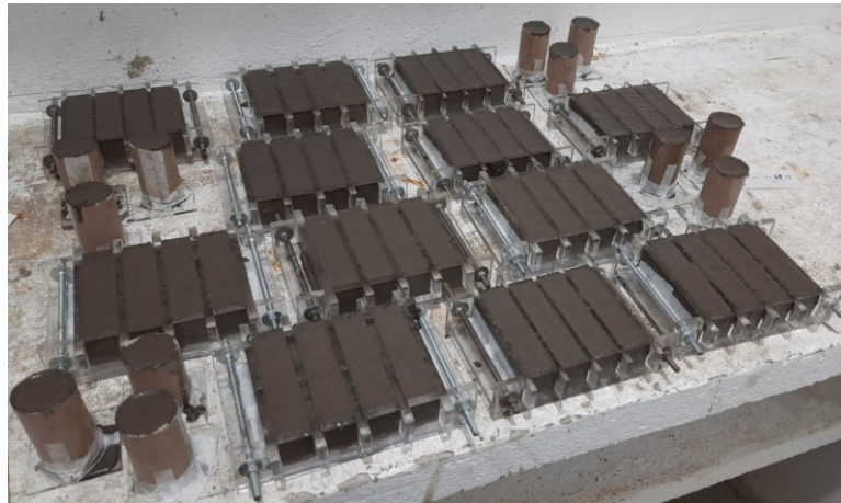
Figure 1 - Specimens being cured in the humid chamber.
