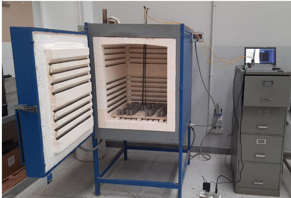
Figure 2 - Experimental setup for the thermal treatments.
