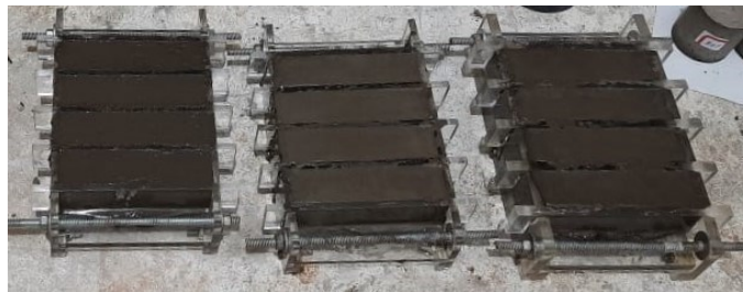
Figure 1 - Production of specimens for compression and bending tests. From left to right: REF-0.72; 0.1NFC-0.72 and 0.2NFC-0.72.
