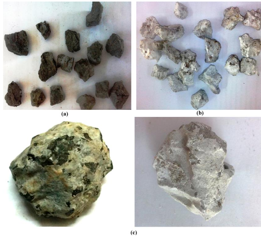
Fig. 2.4 Image showing steel slag aggregates before and after weathering process. (a) Steel slag aggregates before weathering process. (b) Formation of a thin film of calcite on slag aggregates after undergoing weathering process. (c) Enlarged image of steel slag aggregate displaying the presence of calcite coating [191].
