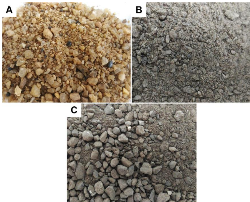
Fig. 4.3 Fine aggregates: (A) quartz sand; (B) gneiss sand; and (C) BOFS sand.
