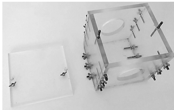
Fig. 3.5 Cubic box made of acrylic for UPV tests [72].
