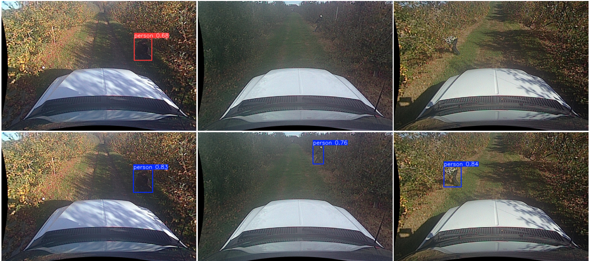
Figure 5.4: Object detection in a rural environment. First line prediction made with original YOLOv8 training and second line with SmartClass.
