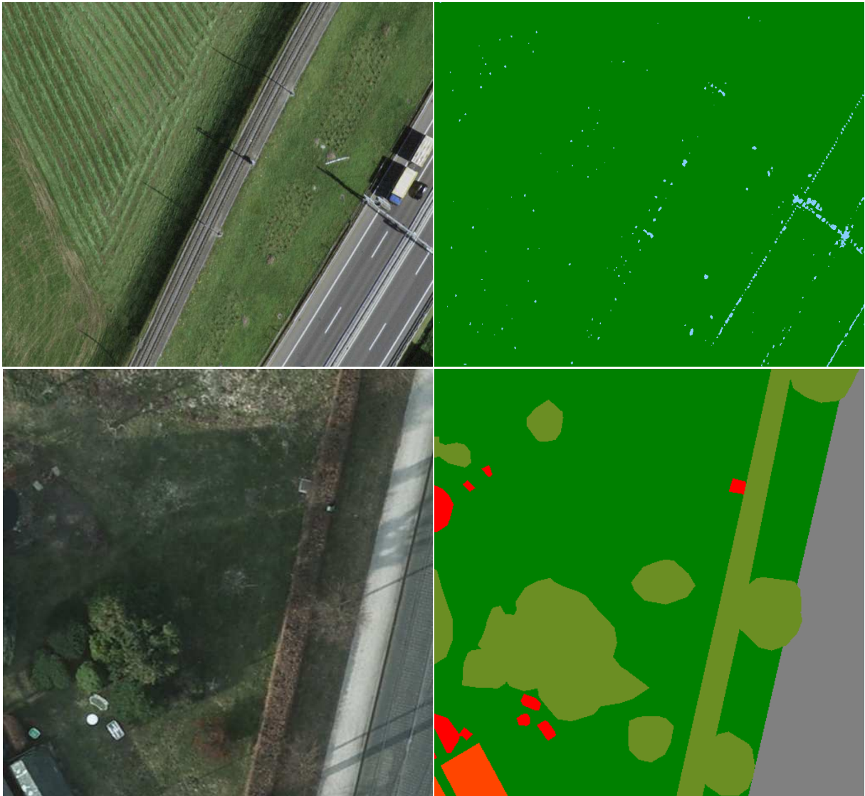
Figure 4.3: Example images demonstrating only the Ground class in the synthetic dataset in the first row. The second row shows the Impervious Surface class for gray ground in the Potsdam dataset.
