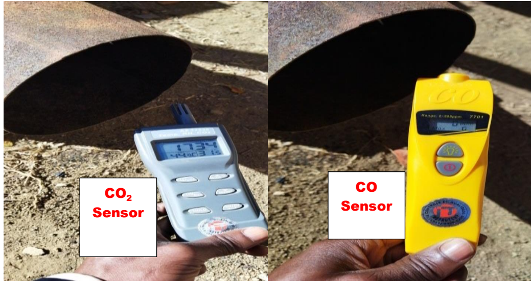
Figure 11: Positioning of the Sensors during the Measurement of Drying air Quality (Source: Author)
