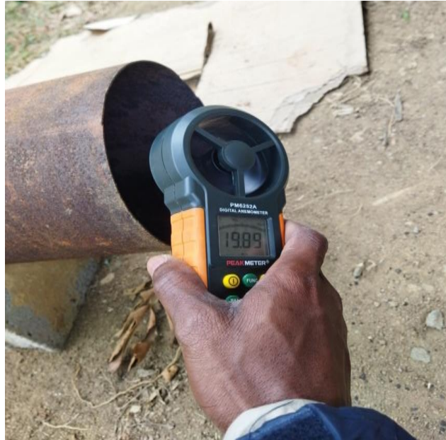
Figure 10: Measurement of the drying air velocity at the air inlet (Source: Author)
