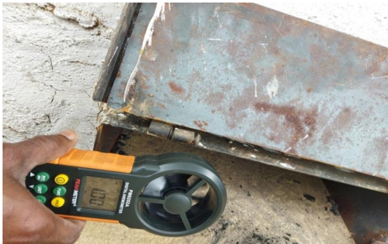
Figure 9: Measurement of the oxidizing air velocity at the primary air inlet (Source: Author)
