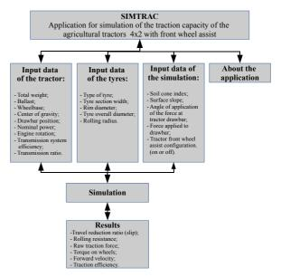
Figure 1. Overall flow diagram for implementation of Simtrac application.
