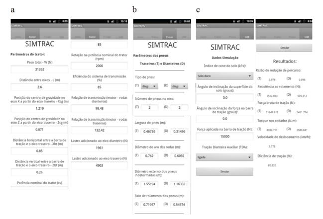
Figure 3. Tabs of Simtrac application implemented with scroll function: a) Trator ('Tractor') tab provides input data of the simulated tractor; b) Pneus ('Tyres') tab provides input data of tyres to be employed in simulation; c) SIM ('Simulation') tab of the Simtrac application with simulation parameters and results.
