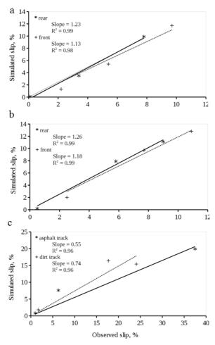
**Figure 4.** Comparison between simulated and observed slip: a) trials performed on asphalt track with front wheel assist on; b) trials performed on dirt track with front wheel assist on; c) trials performed on asphalt and dirt tracks with front wheel assist off.
