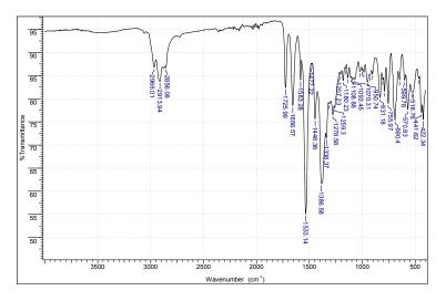
Figure 3. Infrared spectrum (IR) of 7-epiclusianone-copper (liquid film).
