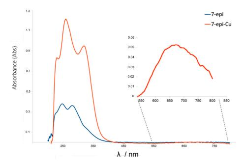
**Figure 4.** UV-VIS spectra of 7-epi (blue) and 7-epi-Cu (red) (0.04 mmol  $L^{-1}$  in methanol) showing the green color absorption of the 7-epi-Cu at 667 nm in the magnified region.
